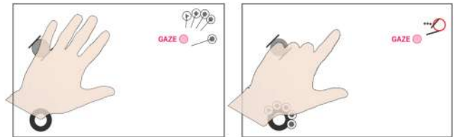
Figure 6. Hand posture can be used to discriminate between widgets in addition to the projected position of the hand or finger. Here, hand posture information is used to select between two widgets that are operated differently.
