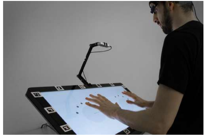
Figure 11. The hardware setup consisting of a touch screen, depth sensor (Leap Motion, attached to the upper screen edge) and eye tracking glasses.
