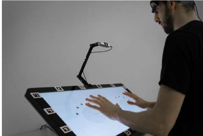
Figure 2: The hardware setup consisting of a touch screen, depth sensor (Leap Motion, attached to the upper screen edge) and eye tracking glasses.
